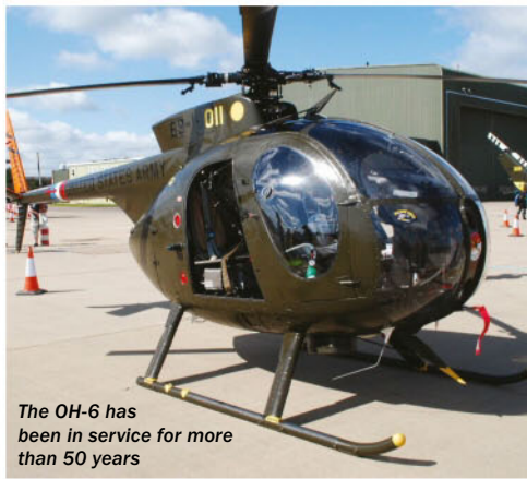
The teardrop or egg-shaped design of the cockpit and crew compartment provided generous space for the pilot and observer/gunner aboard the Hughes
